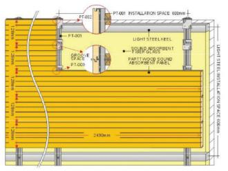
Nero Series Anti-Fungus Acoustic Panel provides superior low frequencies absorption. (Refer to the NRC chart as above). There are two installation menthod, "AT&C" (Aluminium Track&Clip) system and "Nail-On" system. "AT&C" system will provide easy installation and dismantle system.
